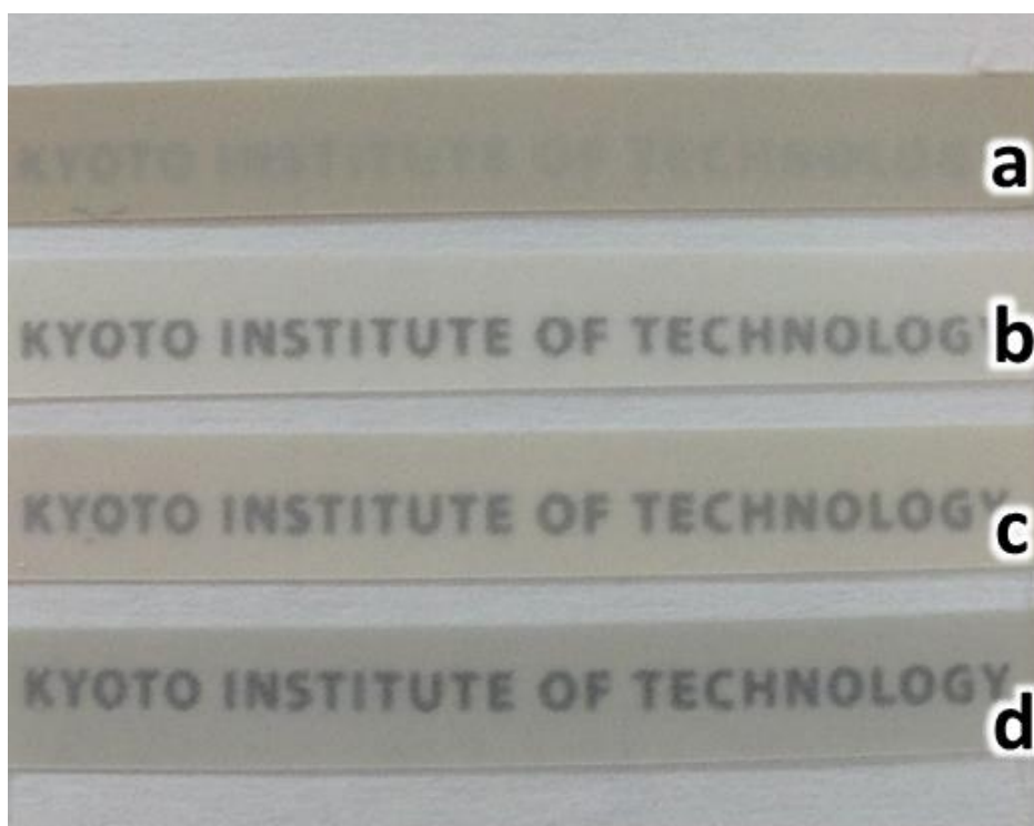
Fig. 2.3. The CNF sheets obtained from the palm pressed fiber (a), empty fruit bunch (b), palm kernel shell (c), and trunk (d).
