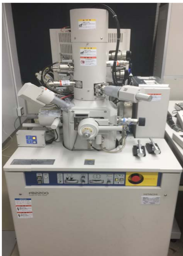
Figure 3.14. Focused Ion Beam system, Hitachi FB 2200 (a), and Scanning Transmission Electron Microscopy observation, Hitachi HD 2700 (b).
