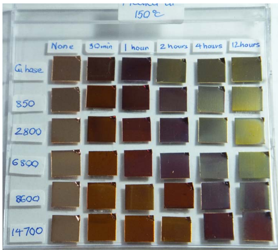
Figure 3.20. Influence of the heat treatment at 150°C for various heating time on the color of copper plate before and after modification with PSt-SHs
