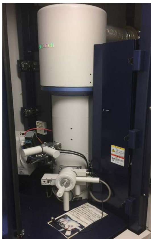
Figure 3.14. Focused Ion Beam system, Hitachi FB 2200 (a), and Scanning Transmission Electron Microscopy observation, Hitachi HD 2700 (b).
