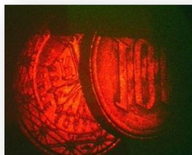
Reconstructed hologram image of coins using photorefractive polymer.
