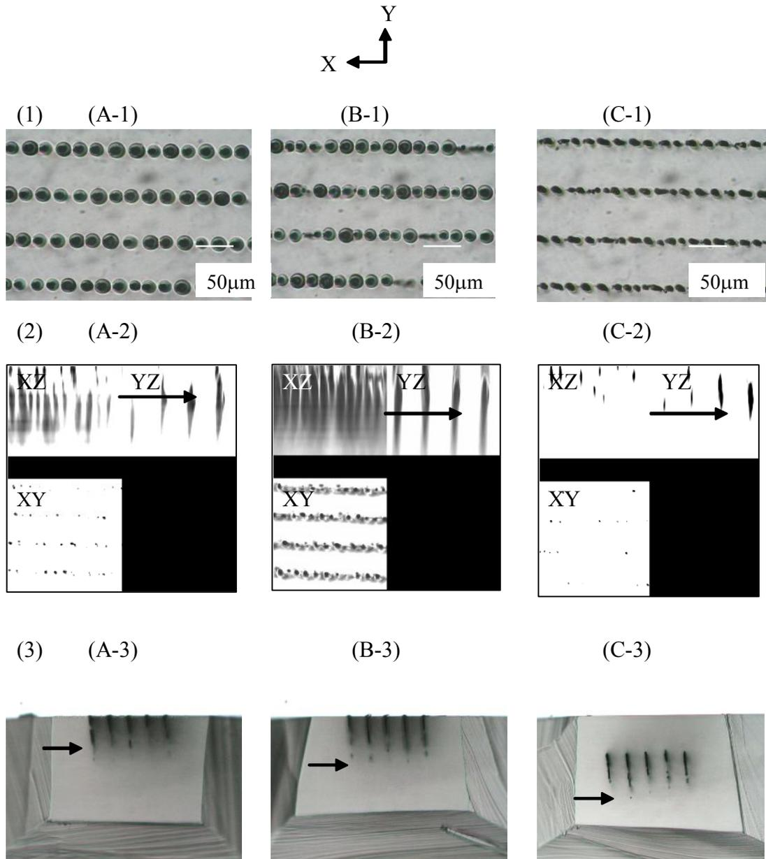
Fig. 2 Micrographs of induced structures by laser irradiation of PC under a condition of constant irradiation energy (100 nJ/pulse) (arrow shows the target depth).
