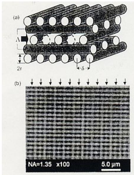
Fig. 11 Schematic of the log-pile structure (a) and optical micrograph of the layer with the defect (top view) in the log pile photonic crystals.
