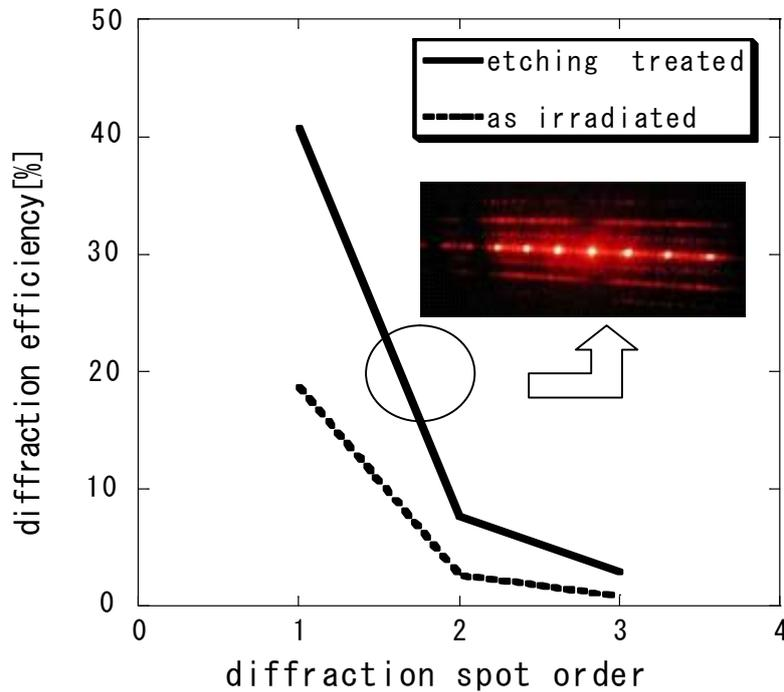
Fig. 4 Refractive diffraction efficiency vs diffraction spot order of Au coated relief grating. Solid line: etched sample. Dotted line: non-etched sample.
