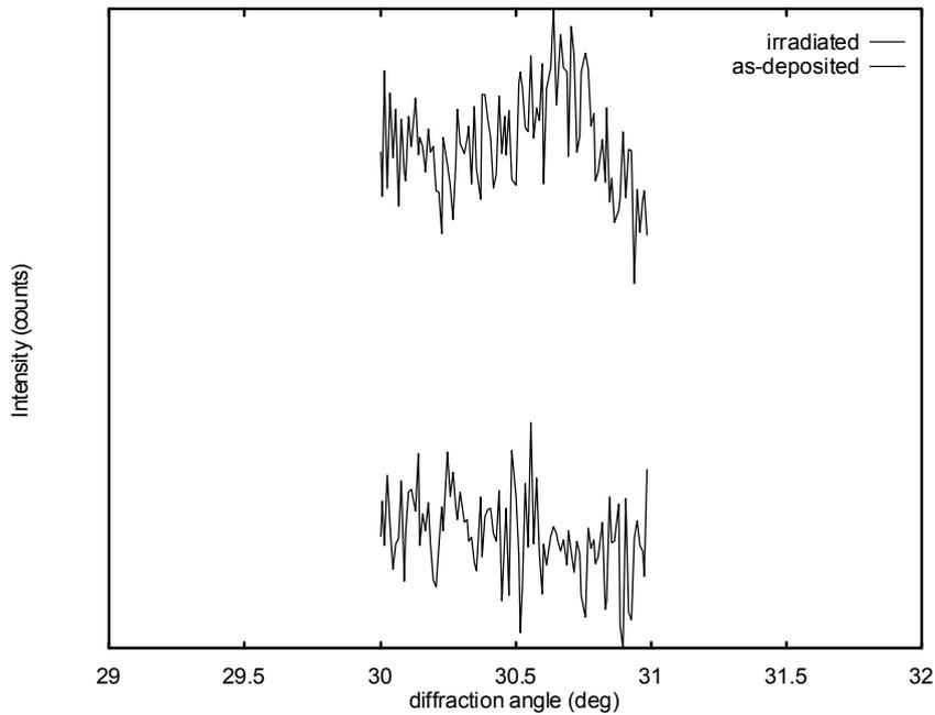
Fig. 2 X-ray diffraction patterns of ( $\text{In}_2\text{O}_3+1 \text{ wt}\%\text{TiO}_2$ ) thin layers.
