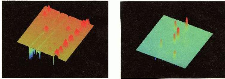
Fig. 2 Optical interference micrograph of volcano-like upheaval on the surface Induced by laser irradiation for higher  $T_g$  polymers : (a) PES and (b) PMMA.
