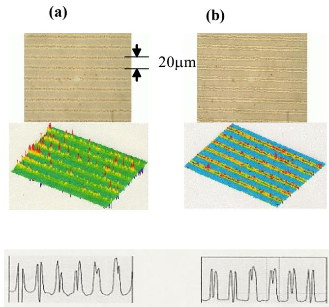
Fig. 1 Optical interference micrographs of relief grating structures induced by femtosecond laser pulses. (a) Irradiated non-etched sample. (b) Irradiated etched sample.
