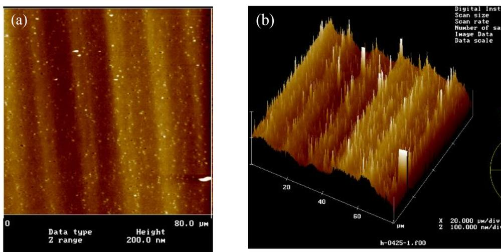
Fig. 8 AFM image of cross-section of irradiated p-(MMA/EA-BA) block copolymer (PMMA; 70 wt%).
