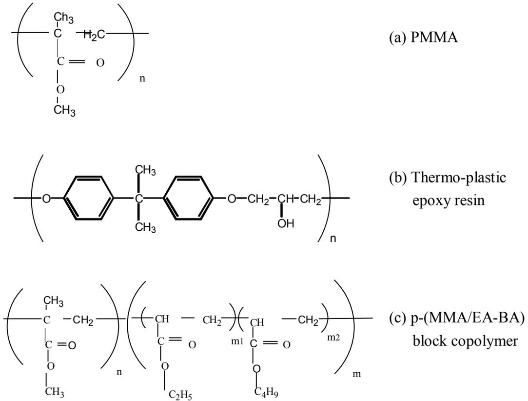
Fig. 1 Structural formulae of polymers used in this study.
