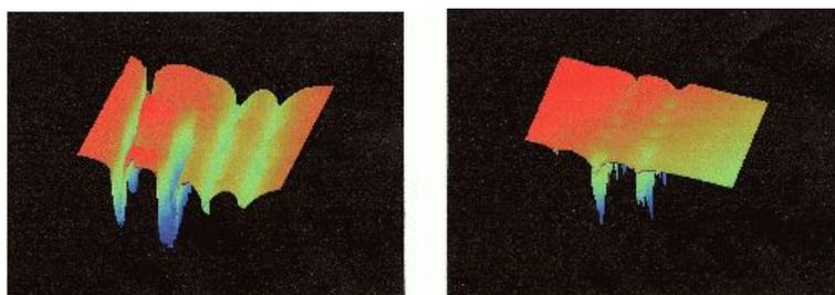
Fig.1 Optical interference micrograph of caves and channels on the surface induced by laser irradiation for lower  $T_g$  polymer: (a) olefine gel and (b) acrylic adhesive.
