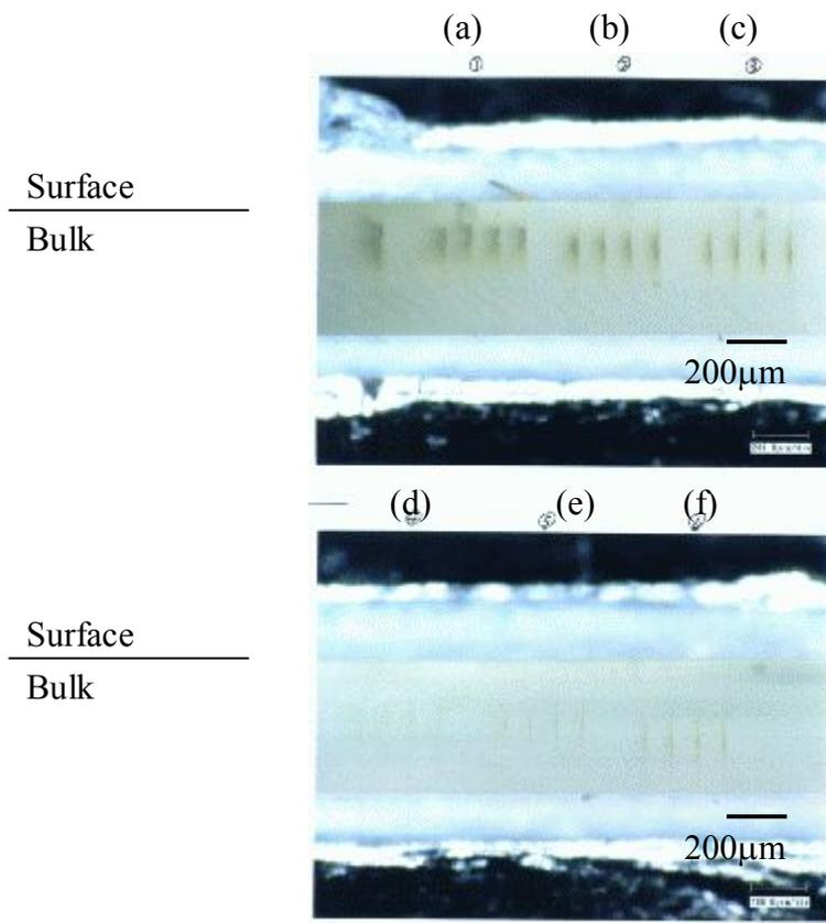
Fig. 5 Optical micrograph of stripe-like structure induced by laser irradiation for PMMA/EA-BA copolymer. (a) 30  $\mu\text{m}$  400 nJ/pulse (b)30  $\mu\text{m}$  300 nJ/pulse (c) 30  $\mu\text{m}$  185 nJ/pulse (d) 30  $\mu\text{m}$  125 nJ/pulse (e) 50  $\mu\text{m}$  125 nJ/pulse (f) 80  $\mu\text{m}$  125 nJ/pulse. (depths are target depths)
