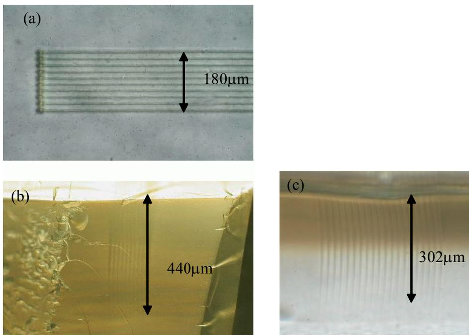
Fig. 2 Optical micrographs of structures induced in PMPS block and PMPS cast film. PMPS block: (a) front view. (b) cross-sectional view.
