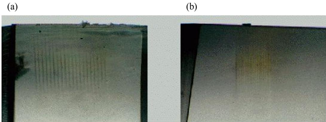
Fig. 6 Optical micrograph of diffraction grating ( $N_G=20$ ).
