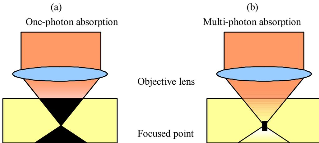
Fig. 4 Schematic of absorption regions for one-photon absorption (a) and for multi-photon absorption (b).
