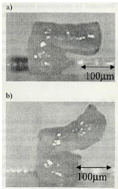
Fig. 13. (a) Optical microscopy image of a micro-cantilever in water prior to UV irradiation. The micro-cantilever was fabricated on a fused silica substrate. (b) Optical microscopy image of the micro-cantilever in water after UV irradiation. The micro-cantilever was irradiated with UV light through the fused silica substrate.
