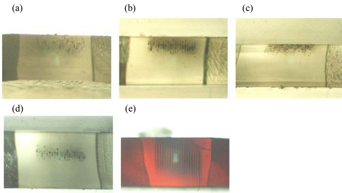
Fig. 5 Optical micrograph of structures induced by laser irradiation for PMMA. (a) PMMA without dye (b) DPA doped PMMA (c) Anthracene doped PMMA (d) DBA doped PMMA (e) DR 1 doped PMMA.
