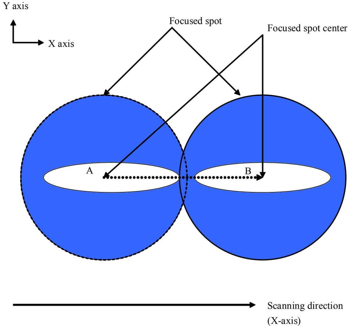
Fig.5 Schematic of the formation of micro-cracks and scanning of focused spot (Open ellipse are micro-cracks).
