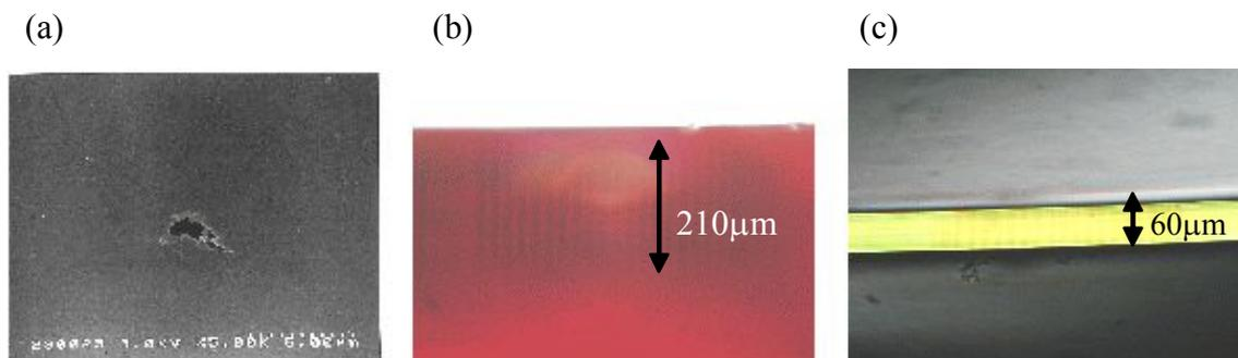
Fig. 4 Optical micrograph of grating structure induced by laser irradiation for PMMA. (a) PMMA without dye (b) Azo dye doped PMMA (c) BTAPVB doped PMMA.
