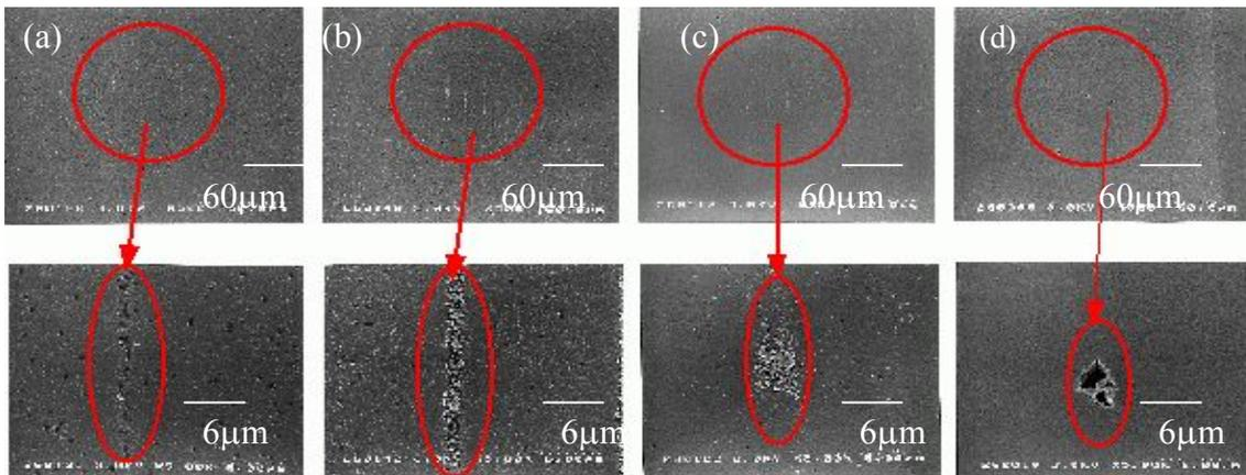
Fig. 7 SEM micrograph of aggregated stripe-like structure induced by laser irradiation for PMMA/EA-BA copolymer (PMMA; 50 wt%). (a) 15 nJ/pulse, (b) 75 nJ/pulse, (c) 140 nJ/pulse, (d) 250 nJ/pulse.
