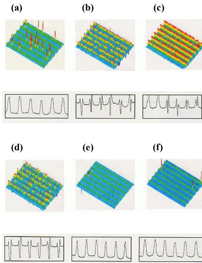
Fig.3 Optical interference micrographs of relief grating structures induced by femtosecond laser pulse under various irradiation conditions. Sample scanning rate;(a) 250  $\mu\text{m/s}$ , (b) 500  $\mu\text{m/s}$ , (c) 750  $\mu\text{m/s}$ . (focused position was on the surface). Focused position; (d) 50  $\mu\text{m}$  above the surface, (e) 100  $\mu\text{m}$  above the surface, surface, and (f) 10  $\mu\text{m}$  below the surface (scanning rate was 500  $\mu\text{m/s}$ ).
