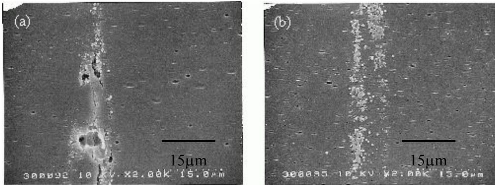
Fig. 6 SEM micrograph of aggregated stripe-like structure induced by laser irradiation for PMMA/EA-BA copolymer (PMMA, 70 wt%): (a) 185 nJ/pulse, 30  $\mu\text{m}$  depth and (b) 125 nJ/pulse, 80  $\mu\text{m}$  depth (depths are target depths)
