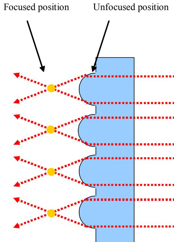
Fig. 5 Schematic of evaluation of micro-lens effect
