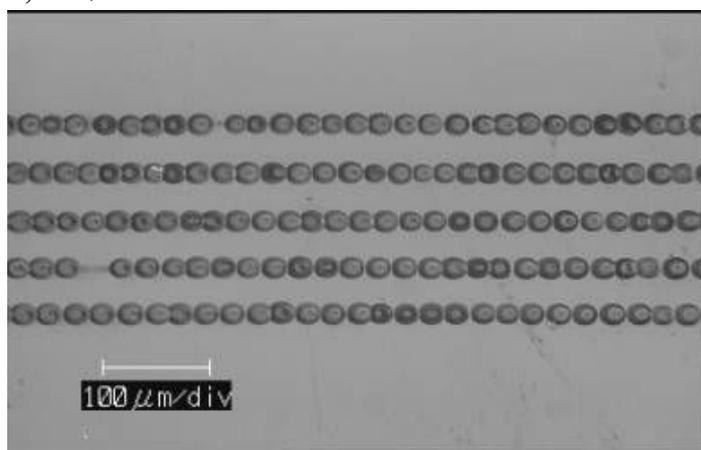
Fig. 2 An optical micrograph of a bell-shaped upheaval of PC.
