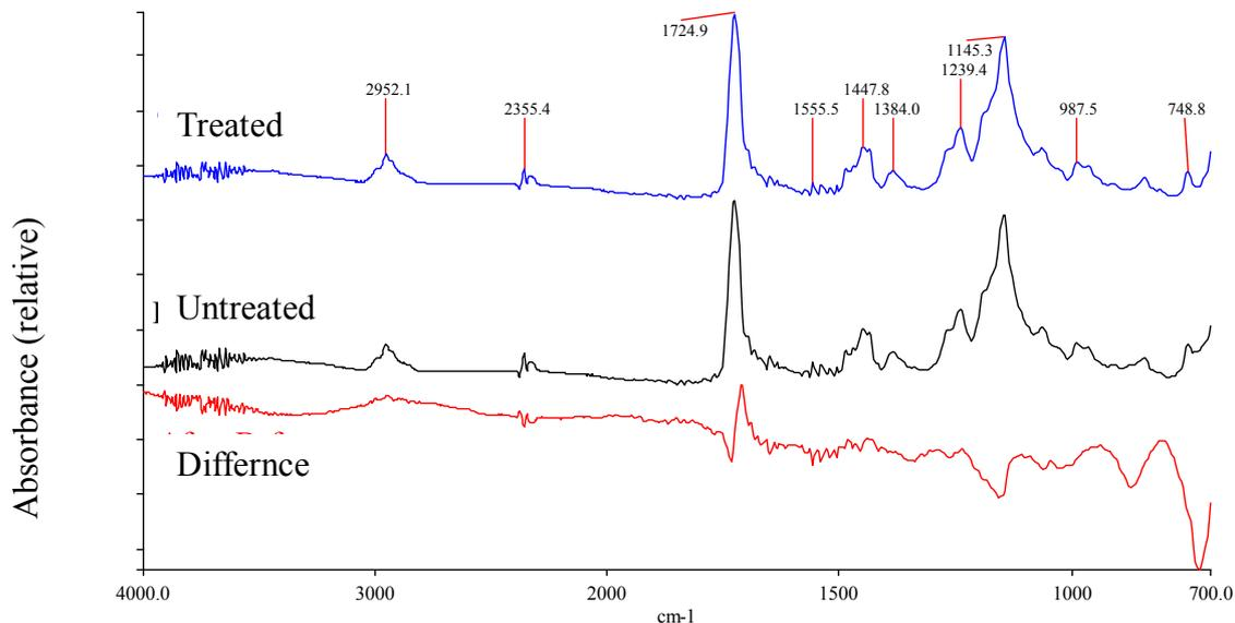
Fig. 9 FT-IR ATR microspectrophotometric spectra of irradiated sample (treated) , un-irradiated sample (untreated) and difference between them for p-(MMA/EA-BA) copolymer (PMMA; 70wt%).
