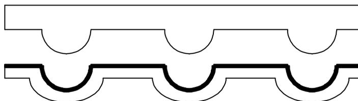
(f) Removal of replicated upheaval structure from the mother mold.
