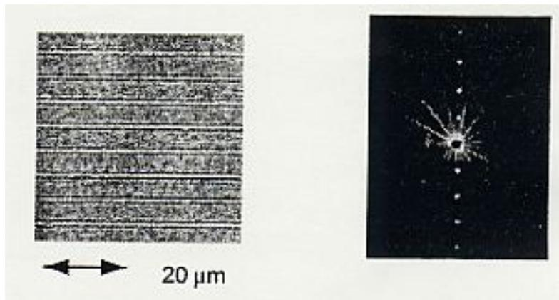
Fig. 10 Diffraction grating formed by ensemble of filament (a) and obtained diffraction pattern.
