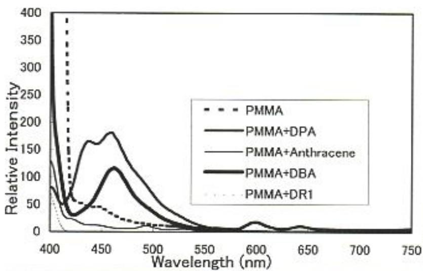
Fig. 7 Fluorescence spectra of PMMA and dye-doped PMMA samples (excitation wavelength: 400 nm).
