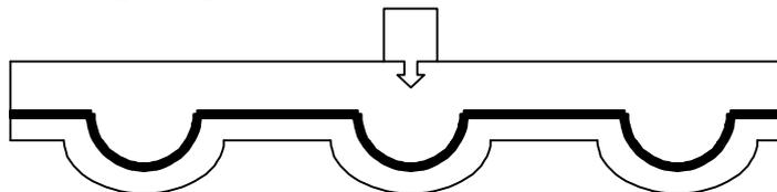
(e) Potting molding material into the mother mold.
