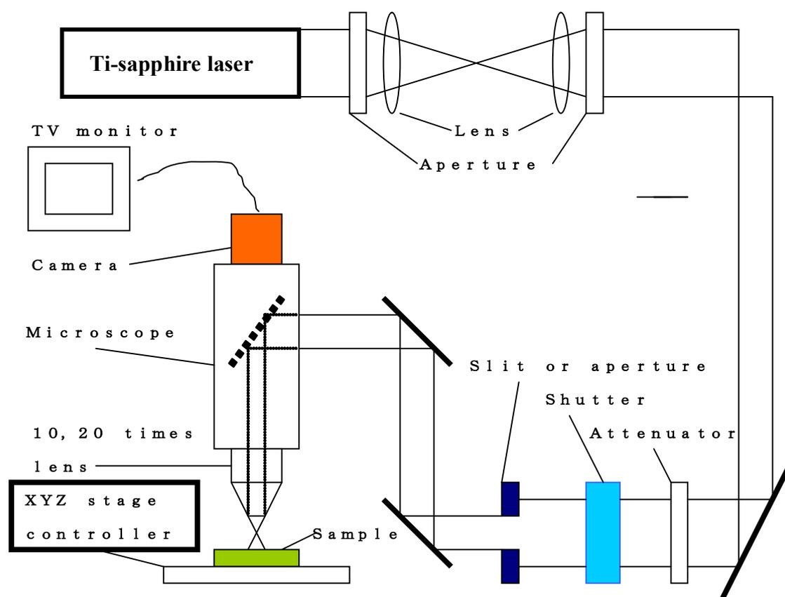
Fig. 1 Schematic diagram of irradiation system using a femtosecond pulse laser.
