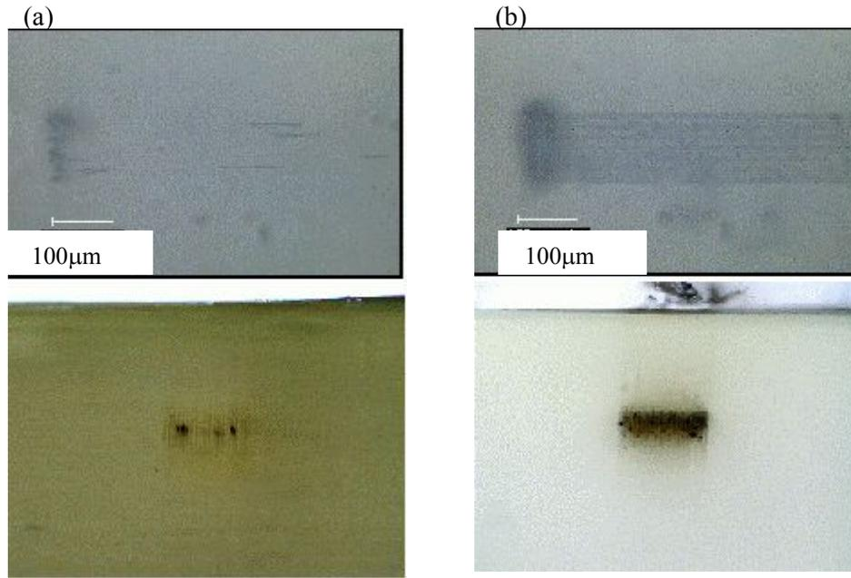
Fig. 8 Optical micrograph of diffraction grating fabricated by single and superimposed lines irradiation of 3 times.
