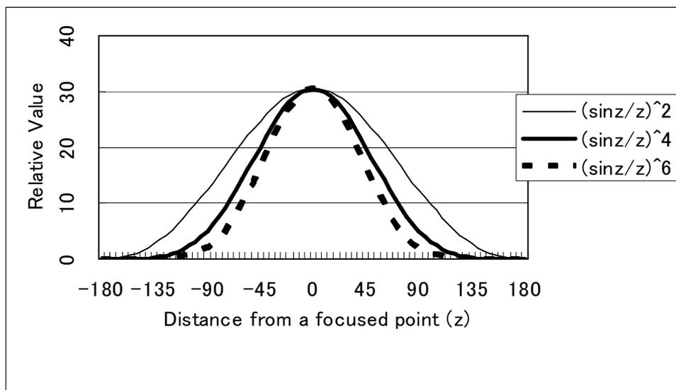
Fig.4. Schematic functional patterns of power density  $(\sin z/z)^2$ , probability of two-photon absorption  $(\sin z/z)^4$  and three-photon absorption  $(\sin z/z)^6$ . In these patterns, relative values are normalized by adjusting same peak value.
