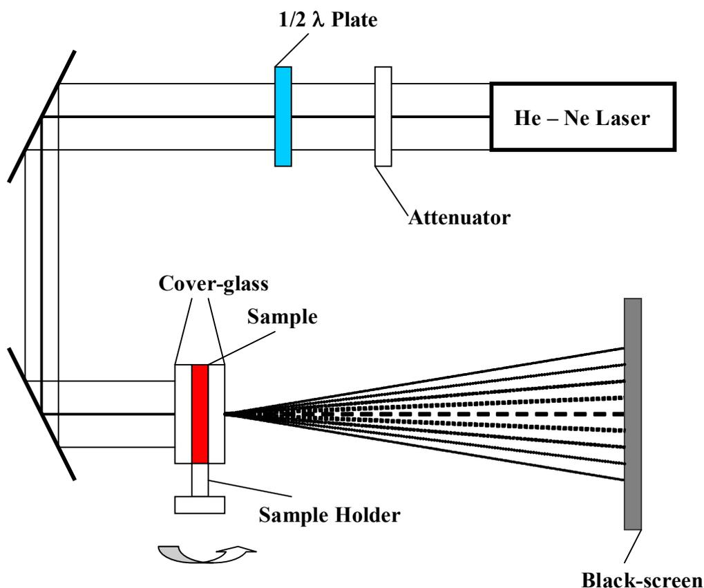
Fig. 4 Schematic diagram of diffraction experiment system.
