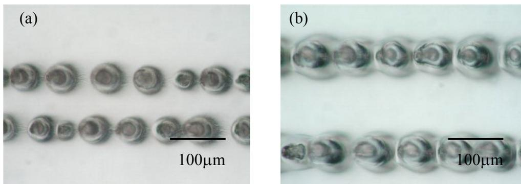
Fig.3 Optical micrographs of upheaval structures of (a) ABSM copolymer and (b) AS copolymer.
