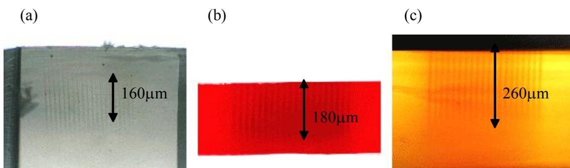
Fig. 3 Optical micrograph of grating structure induced by laser irradiation for p-(MMA/EA-BA) block copolymer. (a) copolymer without dye (b) Azo dye doped copolymer (c) BTAPVB doped copolymer.
