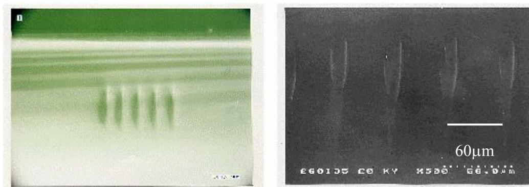
Fig. 10 Micrograph of structure induced by laser irradiation for inorganic glass materials (2500 nJ/pulse, 60  $\mu\text{m}$  target depth).
