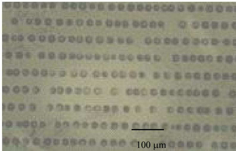
Fig. 6 Optical micrograph of replicated bell-shaped upheaval structure of AS copolymer.
