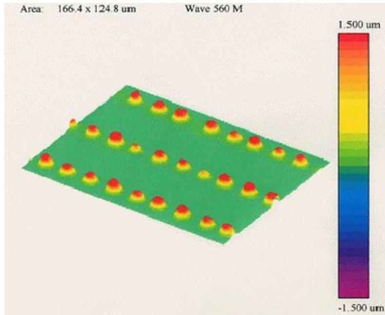
Fig. 1 An optical interference micrograph of an upheaval structure of PC on the surface.
