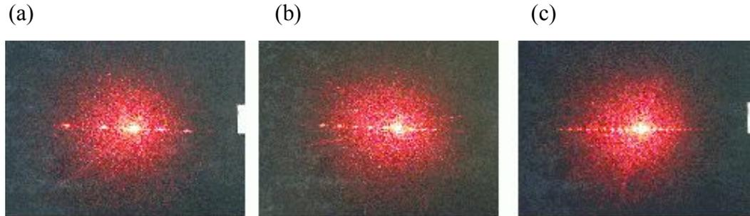
Fig. 2 Diffraction pattern photograph of different  $\Lambda$  for polymer #1. (photo-cross-linker; 1.0 weight part) (a)  $\Lambda=7 \mu\text{m}$ , (b)  $\Lambda=15 \mu\text{m}$ , (c)  $\Lambda=30 \mu\text{m}$
