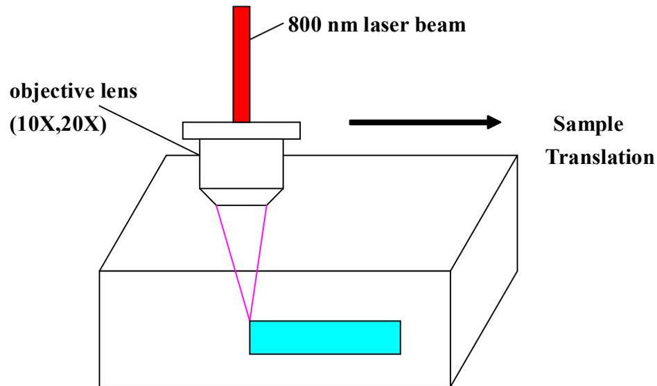
Fig. 2 Line irradiation method. The sample was scanned along the direction perpendicular to the incident laser beam.
