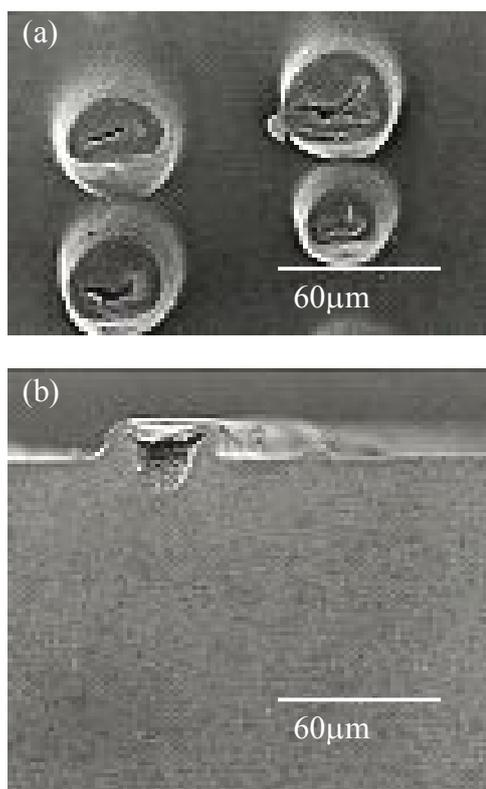
Fig. 4 SEM micrographs of upheaval structure of ABSM copolymer. (a) Front view. (b) Cross sectional view.
