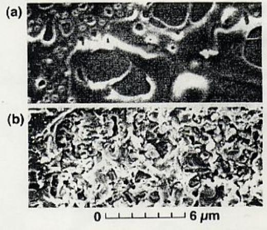
Fig. 2 Scanning electron micrograph of front surface damage of fused silica produced by 1053 nm pulse of duration 900 ps (a) and 500 fs (b).
