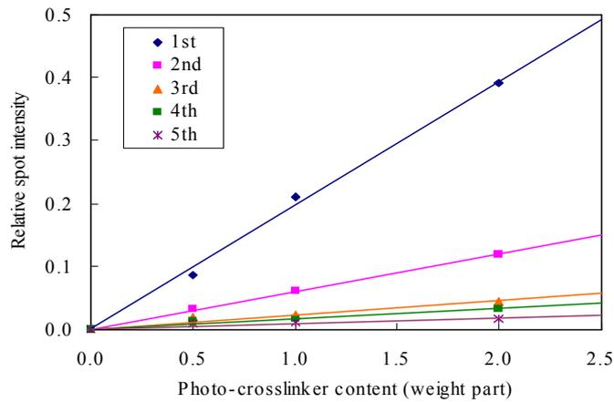
Fig. 4 Relation between diffraction spot intensity and photo-cross-linker content in polymer #1 for each order diffraction.
