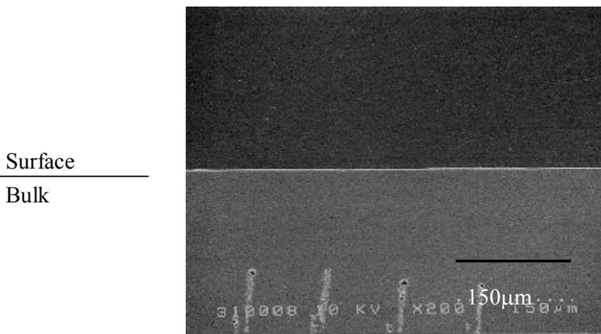
Fig. 4 SEM micrograph of induced voids and cracks by 90  $\mu\text{m}$  depth (depth is target depth) laser irradiation in PC sample.
