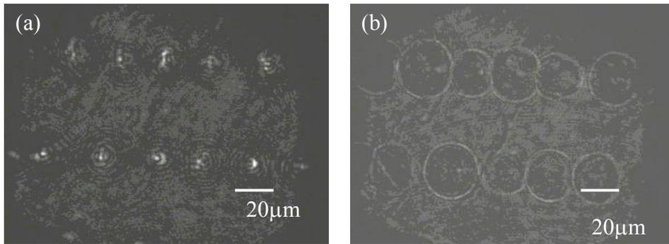
Fig. 8 Micrographs of the transmission images of (a) focused position and (b) un-focused position of replicated AS copolymer micro-lens.
