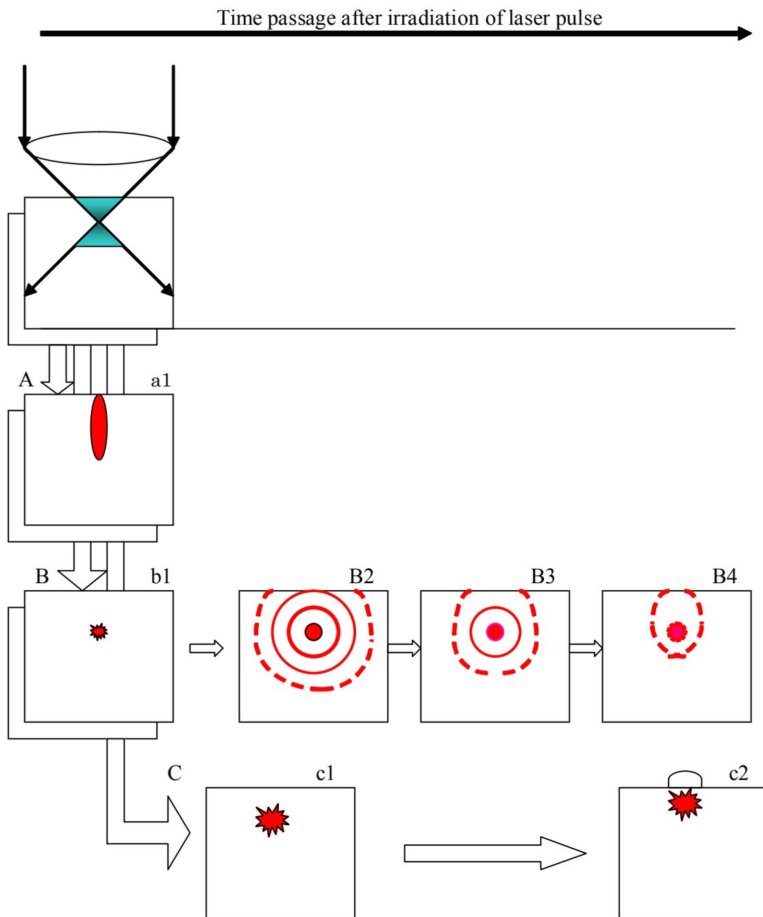
Fig. 6 Schematic representation of induced phenomena by line irradiation of NIR laser pulse in PC at the target irradiation depth 50 μm.
