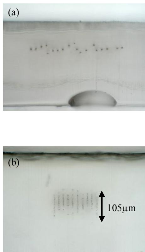
Fig. 4 Optical micrographs of structures induced in (a) Epoxy and (b) PMPS-coated Epoxy.
