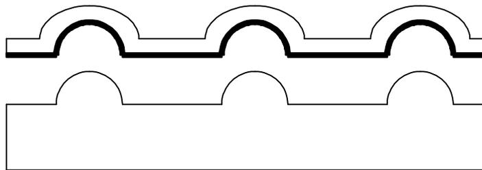
(d) Removal of the mother mold from original bell-shaped structure.
