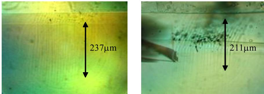
Fig. 3 Optical micrographs of structures induced in PMPS bulk by (a) single line irradiation and (b) superimposed line irradiation for three times.
