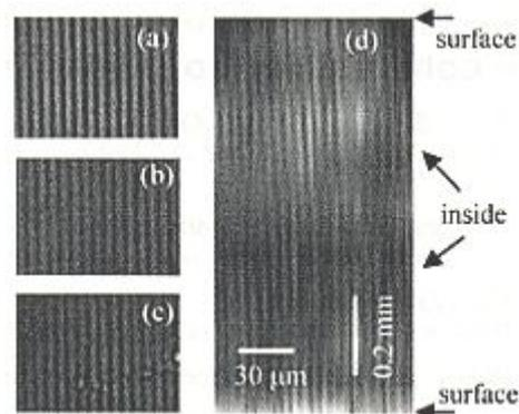
Fig. 14. Optical microscopic photos (a-c) of the photo-induced grating on the top surface (a), in the inner that is 0.4 mm from the top surface (b), and on the bottom surface of the sample (c). The photo on the right (d) is an orthogonal section image of the grating observed using a confocal laser scanning microscope. The horizontal and vertical scale bars represent  $30\ \mu\text{m}$  and  $0.2\ \text{mm}$ , respectively.
