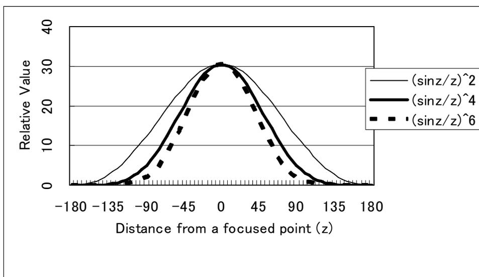
Fig. 6 Relationship between power density, probability of two-photon absorption, probability of three-photon absorption and distance from a focused point (z)
