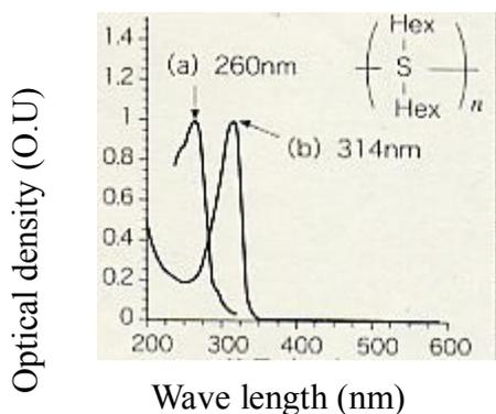
Fig. 5 Absorption spectra of poly (di-hexyl silane).
