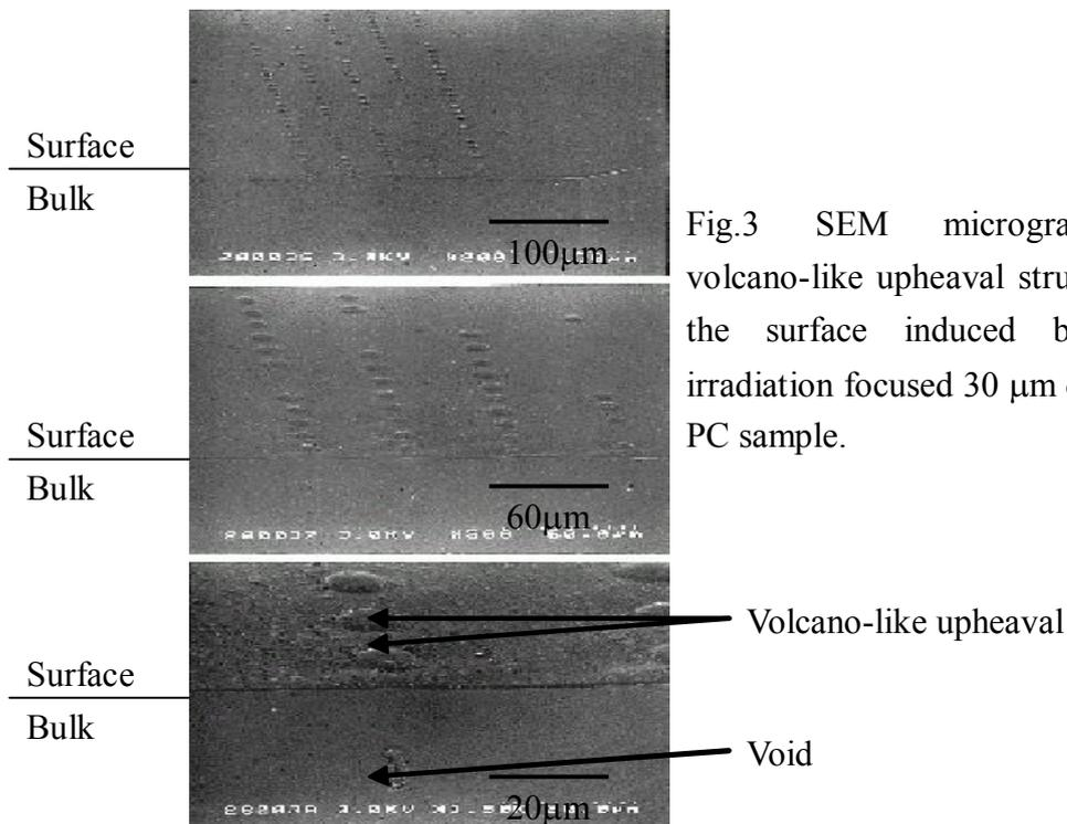
Fig.3 SEM micrograph of volcano-like upheaval structure on the surface induced by laser irradiation focused 30  $\mu\text{m}$  depth. in PC sample.
