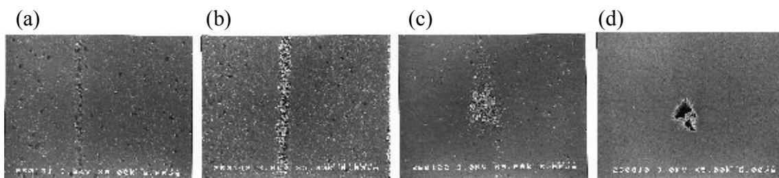
Fig. 1 SEM micrograph of aggregated stripe-like structure induced by laser irradiation for PMMA/EA·BA copolymer (PMMA; 50 wt%).
