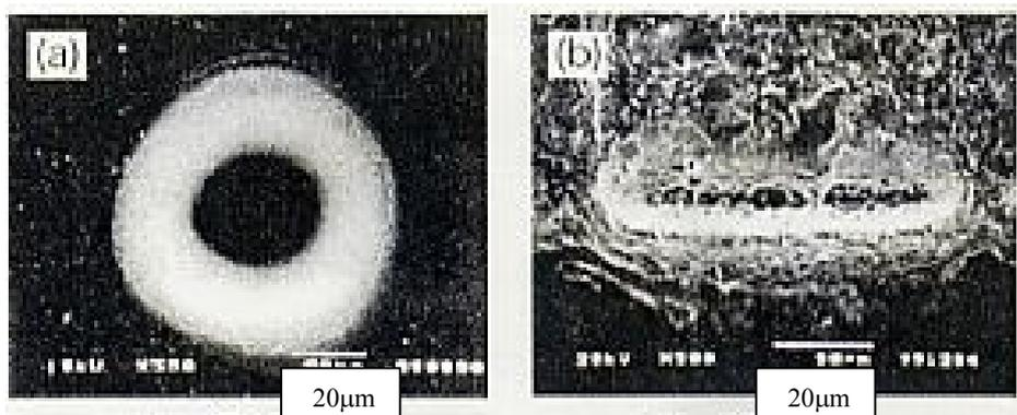
Fig. 3 SEM photographs of after-irradiation on the surface of TiO<sub>2</sub> by Ti-sapphire femtosecond laser pulse with pulse width of 120 fs (a) and KrF nanosecond laser pulse with pulse width of 30 nm (b). irradiated energy, 0.15mJ; number of shots, 3000.
