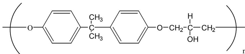
Thermoplastic bis-phenol A type epoxy
