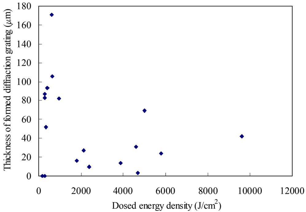
Fig. 5 Relation between thickness of diffraction grating formed and dosed energy density.
