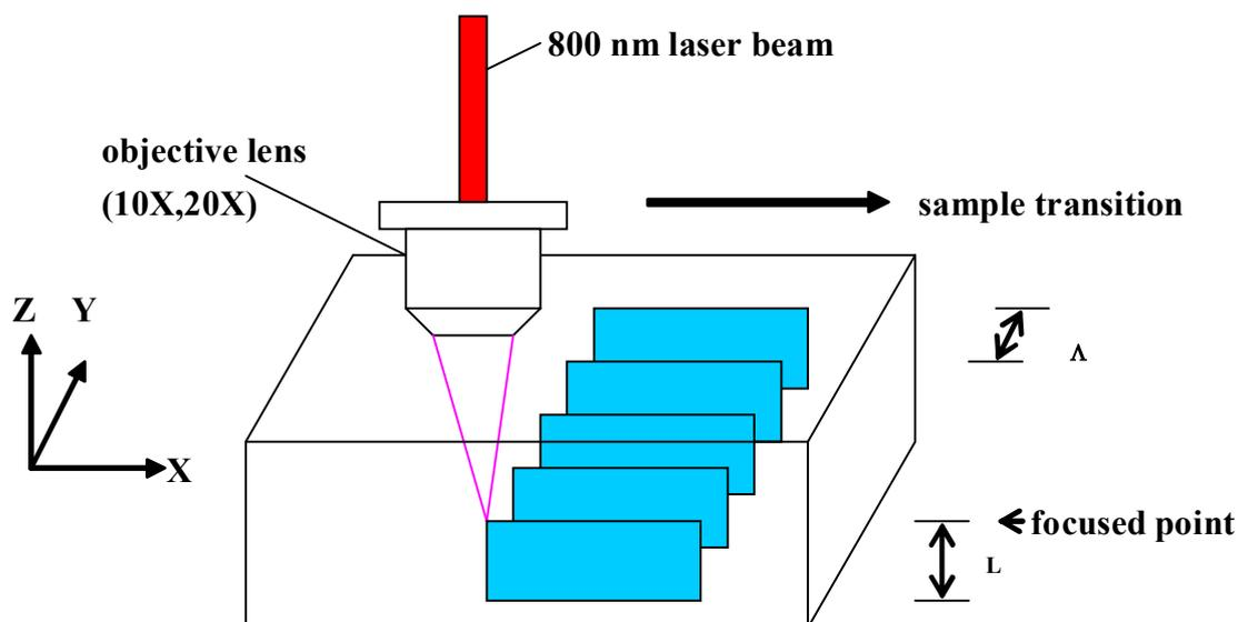
Fig. 3 Line irradiation method in the case of forming a diffraction grating structure.
