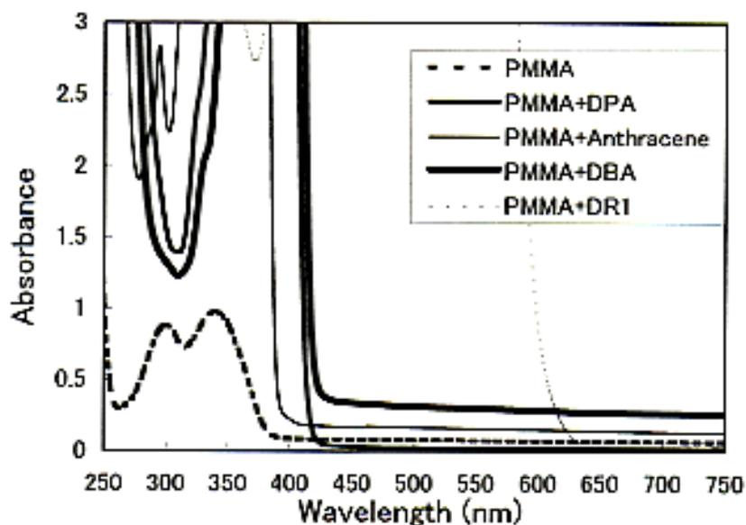
Fig. 6 Absorption spectra of PMMA and dye-doped PMMA samples.
