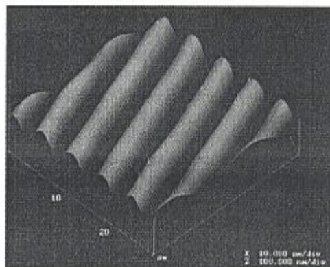
Fig. 15. AFM scans of the photo-induced gratings. The surface modulation of the surface relief gratings is about  $50\ \text{nm}$
