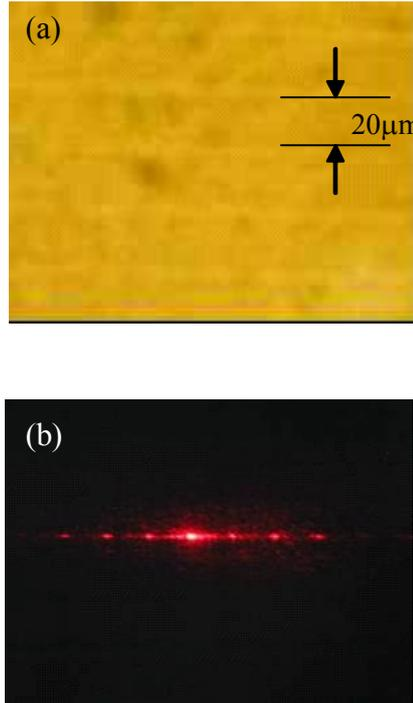
Fig. 5 (a) Optical micrograph of structures induced in PMPS-coated PMMA (front view). (b) Diffraction pattern from the structures.
