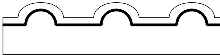
(c) Electrolytic plating of Ni over pre-coated Ni.
