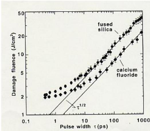
Fig. 1 Observed value of damage threshold at 1053 nm for fused silica (●) and CaF<sub>2</sub>(◆). Solid line are  $\tau^{1/2}$  fits to long pulse results. Estimated uncertainty in the absolute fluence is  $\pm 15\%$ .
