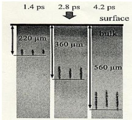
Fig.8 Microscopic sideview of bulk modifications in a-SiO<sub>2</sub> after 100 laser shots, with the laser beam focused at the entrance surface, for three different pulse duration. The energy per pulse was 20 μJ, focus diameter 920 μm<sup>2</sup>, and λ=790 nm.
