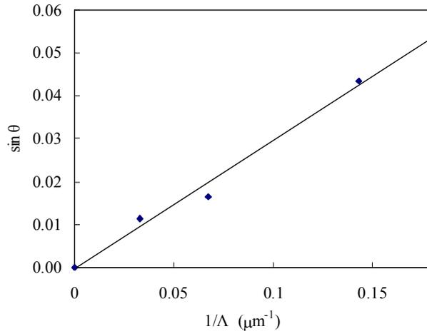
Fig. 3 Relation between distance of diffraction spot and 1/(interval between diffraction grating).
