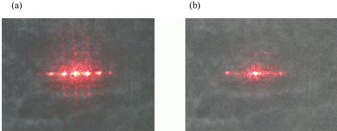
Fig. 7 Diffraction pattern photograph of sample fabricated by the optical condition and with narrowest  $\Lambda$ .
