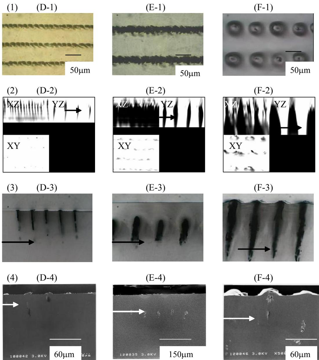
Fig. 3 Micrographs of induced structures by laser irradiation of PC under a condition of constant target irradiation depth (50  $\mu\text{m}$ ) (arrow shows the target depth).
