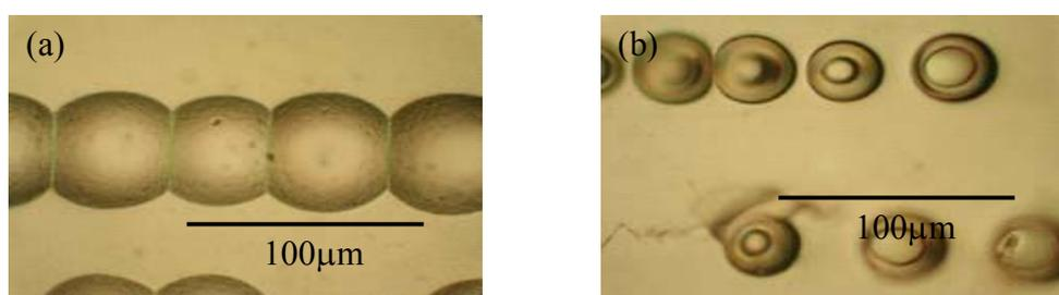
Fig. 5 Optical micrographs of the mother mold obtained by the electroforming process. (a) Front view. (b) Back view.
